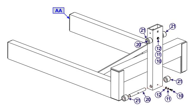
Apply a small amount of anti-seize inside of rollers prior to placing on axle
