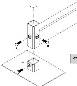
Tighten set screws A & B alternately to push leg securely into corner of leg socket.
