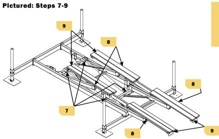
Use a small amount of 'moly' lube on bolt threads through the assembly process.
