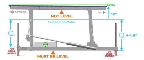
Leveling requires a second person to support the crossmember while making adjustments. If the lift is too heavy for two people, a ratchet strap or winch system will be required to raise/lower the frame corners.
