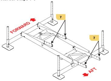
Use a small amount of 'moly' lube on bolt threads through the assembly process.
