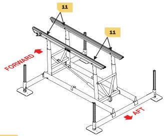
Use a small amount of 'moly' lube on bolt threads through the assembly process.
