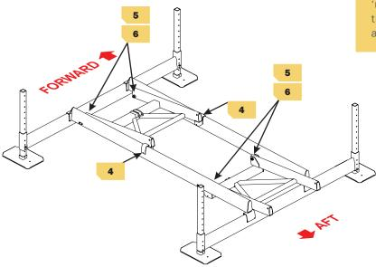
Use a small amount of 'moly' lube on bolt threads through the assembly process.
