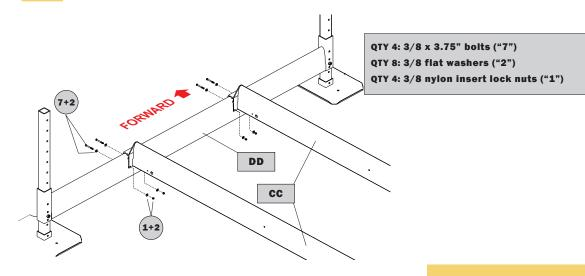
Assemble lift on level ground and adjust legs so that lift base frame is level during lift assembly.
