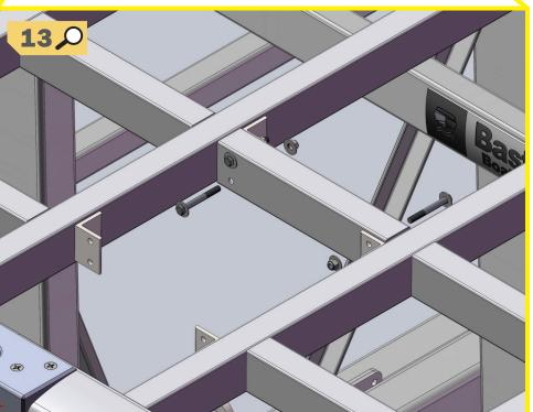
Each connector tube requires four bolts, four lock nuts and eight washers as shown.
