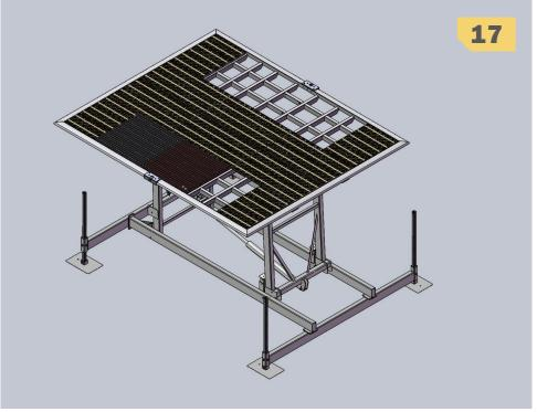
Lay the central tube in the groove that runs down the center of the lift. The side with the beveled holes should be on top.
