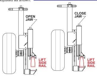
THE JACK HAS 15" OF ADJUSTMENT. THE CENTER POST HAS 12" OF ADJUSTMENT, FOR A TOTAL OF 27" OF ADJUSTMENT.
