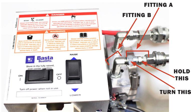
6. Reconnect the hydraulic hose line separated in step 21.
