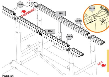
Placement may need to be modified based on watercraft draft and weather conditions.
