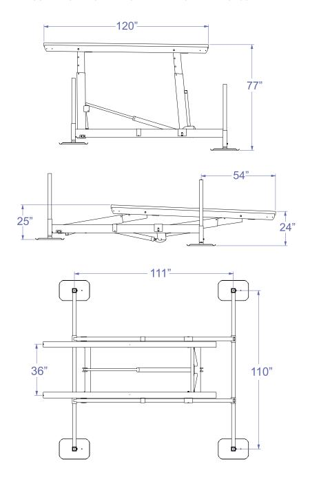
**IMPORTANT:** The leveling process must be completed to ensure stability of the lift frame and Over-Center safety lock.
