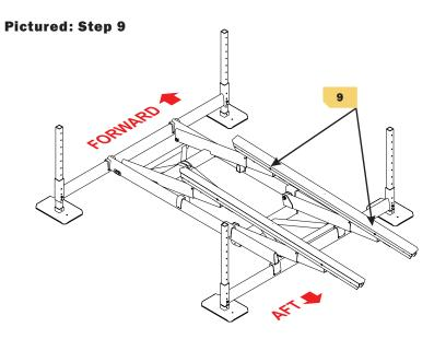
Model 4.5k37 only: Remove black bunk bushings and replace with shorter white bushings before proceeding with this step.
