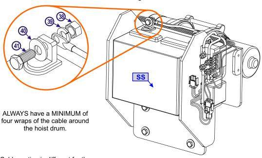
Cable routing is different for the manual hoist
